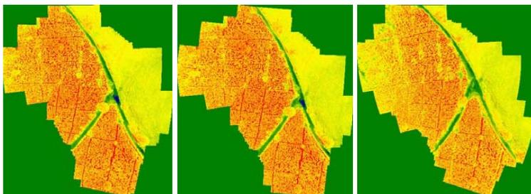
Figure 23. NDVI with #19 Filter and AWB 0.54,1 Configuration
