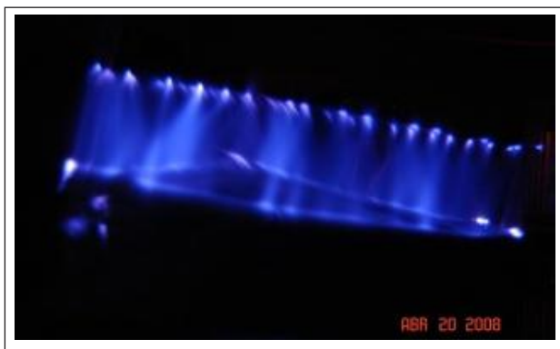
Figure 3. Prototype levitating, power supply 21 kV.
